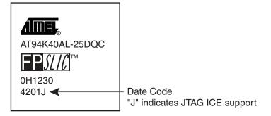
Figure 1. FPSLIC Device Date Code with JTAG ICE Support
