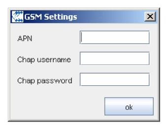
In order to send data via GSM GPRS/EDGE network, camera must have the access point address. "Chap username" and "Chap password" is not required in most of networks.
