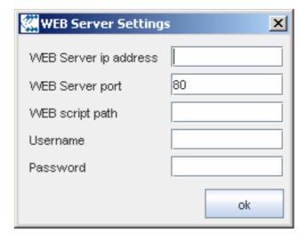
These parameters are set only if the pictures will be sent to server WEB script or to Observation Post software on the PC with static IP address.
