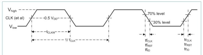
Fig 8. External clock drive and AC test timing reference points of I2C\_SDA, I2C\_SCL, and RST\_N (see <u>Table</u> note [3] and Table note [4]) in open drain mode
