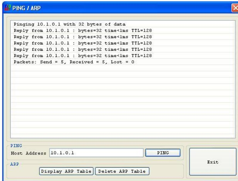
Figure 3-5 ping test when the IP address is 10.1.0.1
