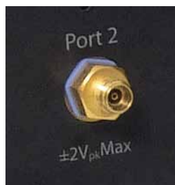
The SPARQ utilizes high-precision 2.92 mm connectors—these can be mated with precision SMA connectors.
