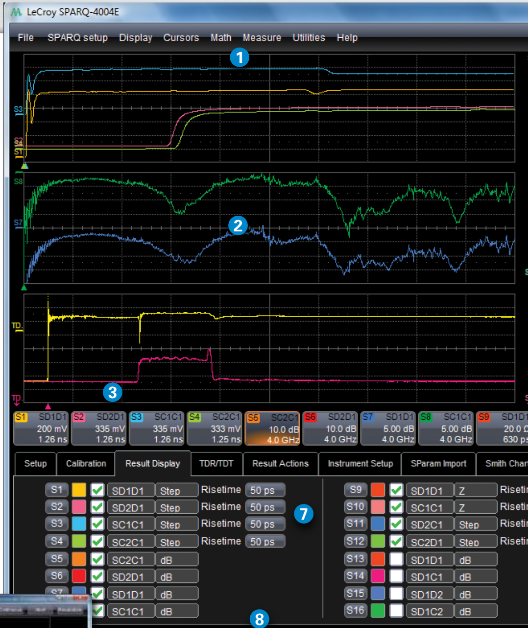
The SPARQ signal integrity network analyzer displays time and frequency domain measurement results simultaneously.
