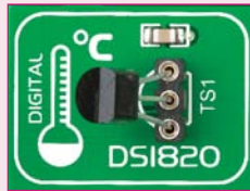
Figure 20-2: DS1820 correctly placed in socket
