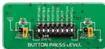
Figure 6-5: Button press level DIP switch (tri-state)
