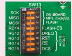
Figure 14-2: Enabling audio codec communication lines
