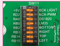
Figure 21-3: Enabled SW11.4 DIP switch
