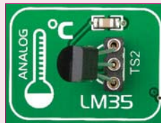
Figure 21-2: LM35 correctly placed in socket
