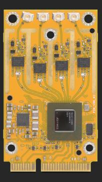
Mini Pini is an 802.11ax Wi-Fi 6 radio module for ultra-high speed enterprise connectivity. Device comes out in three different versions:
