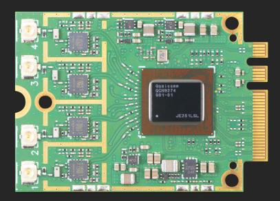
Discover the Noni, a state-of-the-art WiFi7 radio module in a compact M.2 A+E form factor. Powered by Qualcomm's QCA9274/QCA6274 chipsets, Noni operates on the IEEE 802.11be standard with speeds over 11 Gbps in 4x4 MIMO or split 2x2 + 2x2 configurations. It supports up to 320 MHz channel sizes and advanced 4K QAM modulation, enhancing efficiency and connection quality.
