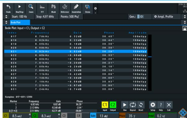
The measurement results table provides detailed information about each measured point (frequency, gain and phase shift). When using markers, the associated row of the result table is highlighted. For reporting, quickly save screen shots, table results, or both to a USB device.
