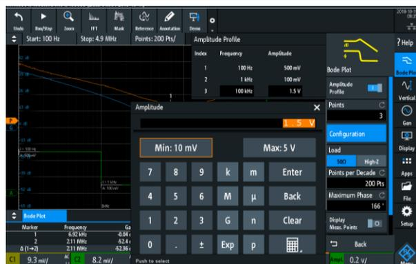
Profiling the amplitude output level of the generator. This is helpful to suppress the noise behavior of your DUT when measuring control loop response or power supply rejection ratio and to improve the signal-to-noise-ratio.
