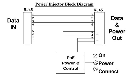
**Description of LED Functions for Power Injector**
