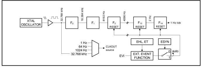
Setting the clock and calendar values synchronous to an External Event detection on EVI pin:
