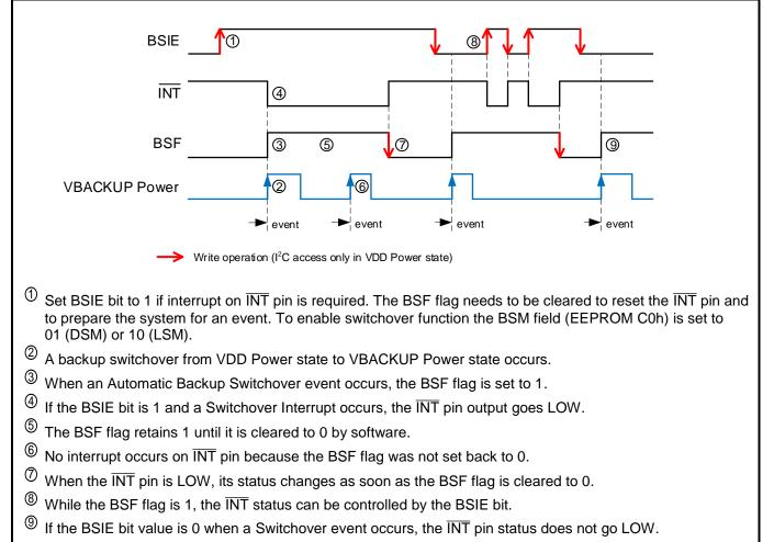
Diagram of the Automatic Backup Switchover Interrupt function:
