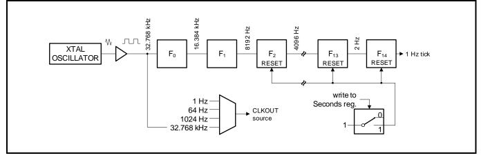
Setting the clock and calendar values using the reset function when writing to the Seconds register:
