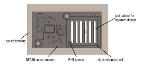
Figure 6: Exemplary aperture design with a slot pattern above the sensing elements of the SFA30 sensor module.
