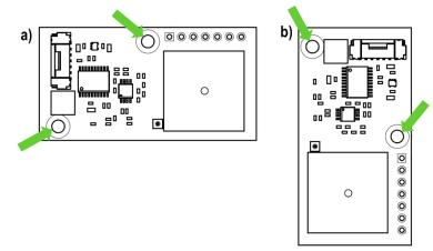
Figure 5: Mechanical mounting (two mounting holes indicated by green arrows) and recommended orientation of SFA30 sensor module with the Molex connector facing (a) sidewards and (b) upwards.
