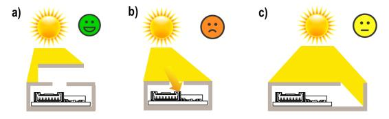
Figure 4: Sensor protection from sunlight (connector view). (a) Good protection and (b) bad protection from incoming sunlight. (c) Good protection from sunlight, however, at the cost of bad coupling to ambient and a large dead volume.
