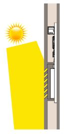
Figure 8: Cross-sectional view: sun protection through an angled aperture design.
