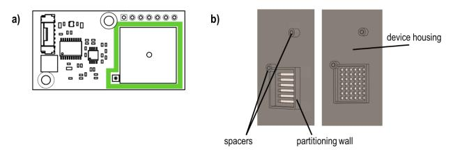
**Figure 7**: Sealing and shielding around the sensing elements of the SFA30 sensor module to prevent or at least reduce the impact from local environmental conditions inside the device on the sensing performance(a) Top view: area marked in light green to be used for sealing or shielding purposes and (b) Internal view of device housing: exemplary implementation of partitioning walls surrounding the sensing elements including two possible aperture designs.
