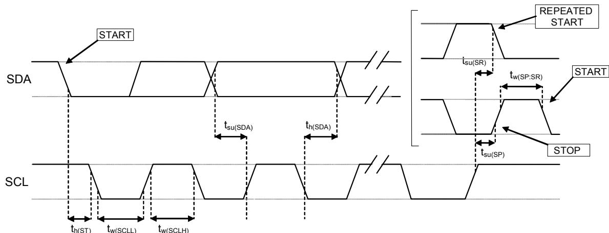
**Note:** Measurement points are done at 0.3·VDD and 0.7·VDD for both ports.
