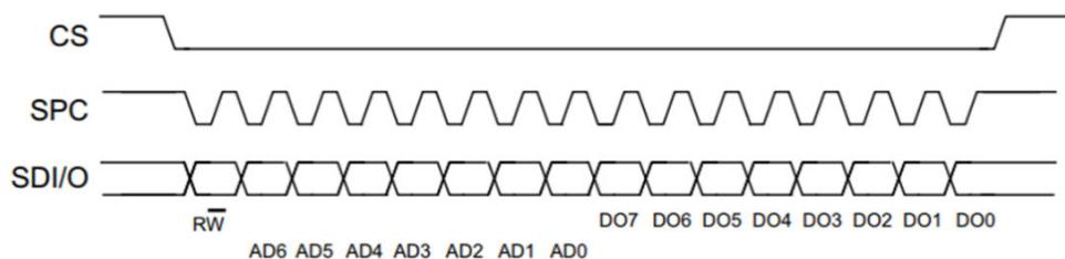
The SPI read command is performed with 16 clocks pulses:
