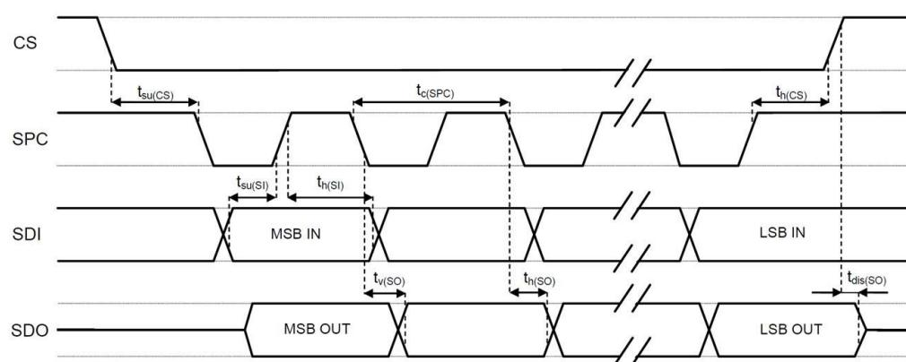
Note: Measurement points are done at  $0.3 \cdot V_{DD}$  and  $0.7 \cdot V_{DD}$  for both ports.
