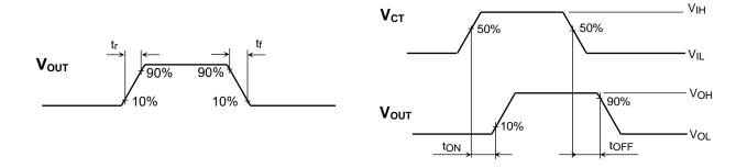
Figure 1 t<sub>r</sub>, t<sub>f</sub>, t<sub>ON</sub>, t<sub>OFF</sub> Waveforms
