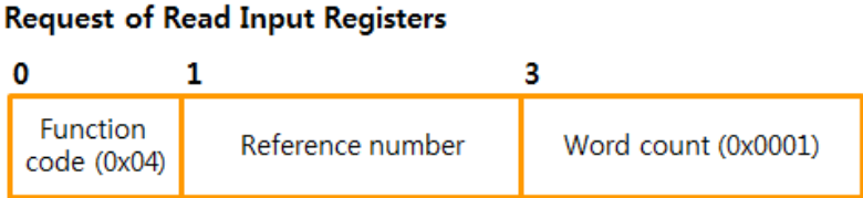
Figure 4-11 request of read input registers
