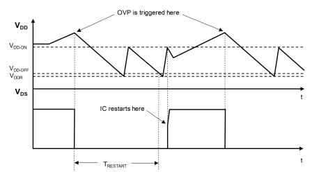
Figure 26. OVP timing diagram
