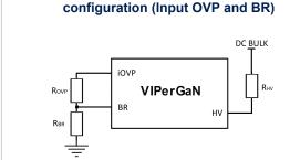
Figure 28. Brown-In/Out and input OVP: external
