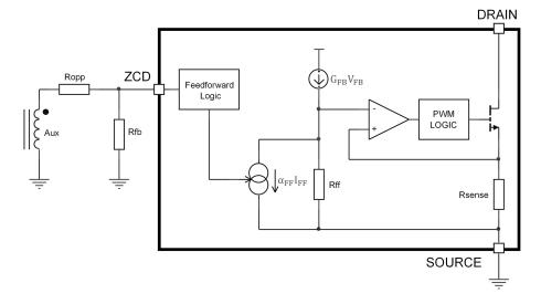
During GaN's on-time the current sourced from the ZCD pin through the R<sub>OPP</sub> resistor is mirrored inside the "Feed-forward Logic" block to provide a feed-forward current I<sub>FF</sub>, proportional to the input voltage according to the formula:
