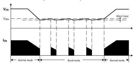
Figure 14. Burst-mode operation
