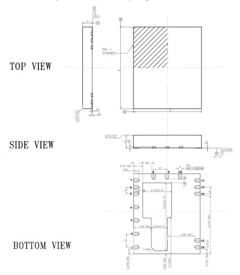
Figure 35. QFN 5x6 narrow package information
