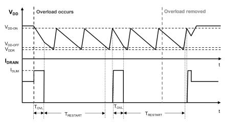
Figure 25. Timing diagram of OLP protection
