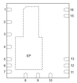
Figure 2. Connection diagram (top view)
