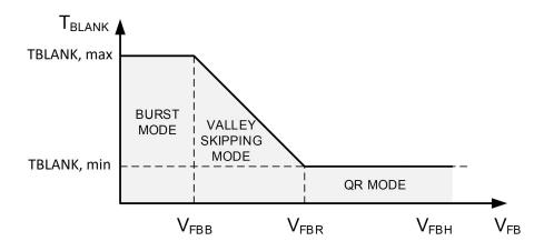
Figure 12. Frequency limits and modes of operations
