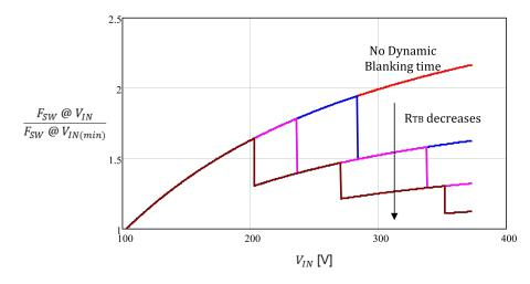
Figure 18. Typical normalized switching frequency variation over input voltage range
