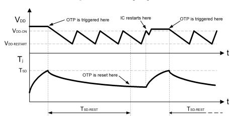
Figure 32. OTP timing diagram
