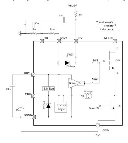
Figure 11. High voltage start-up generator: internal schematic and pin configuration
